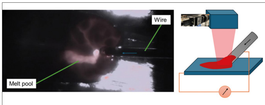
Figure 8: Example of a coaxial camera picture and sketch of the conductance measurement system.
