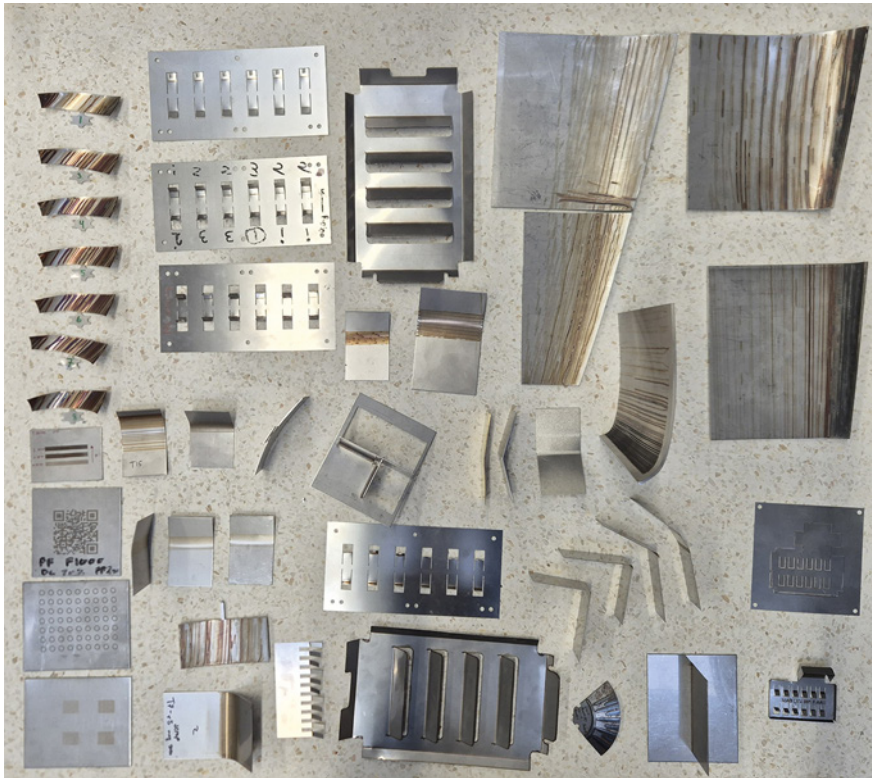
Figure 1: Various sheet metal parts manufacturing with laser integrated manufacturing.
