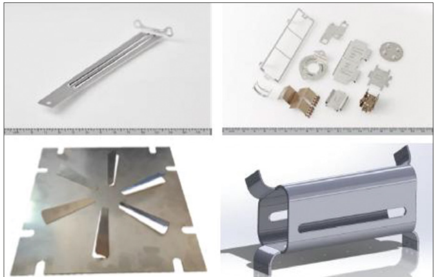
Figure 12: Examples of integrated laser processing approach applications.
